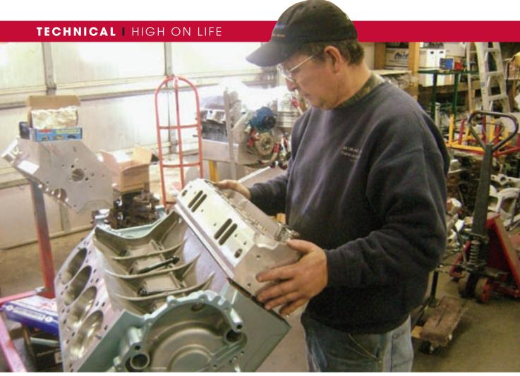
By raising the intake ports on their High-Port heads, Kauffman Racing Equipment was able to straighten out the intake port and dramatically improve airflow to the back of the valve. Better flow is essential to making power, and these heads can flow: how's 630- horses on a pump-gas 467-inch Pontiac sound to you?
