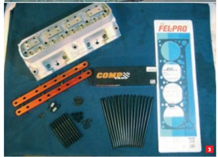
the valve and ultimately into the cylinder. In "stock" trim, straight out of the box, the high-port heads flow approximately 330 cfm — a dramatic improvement compared to low-200 figures for most stock Pontiac heads. Or put in layman's terms: on a .030"-inch over 455 (463 cid), the high-port heads helped it develop 700 horsepower and an amaz-
