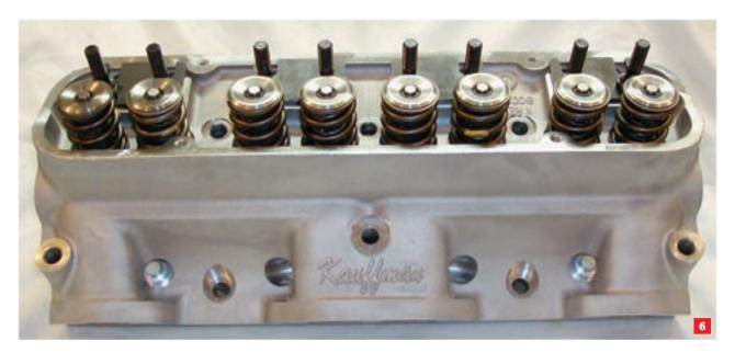
6 In fully-assembled form, the heads are ready to bolt on. The stud girdle kit is available as an option, but is recommended.
