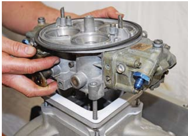
A Holley 1050 Dominator carb is mated to the Edelbrock Victor intake's 850-cfm carb-style flange via an adaptor.
