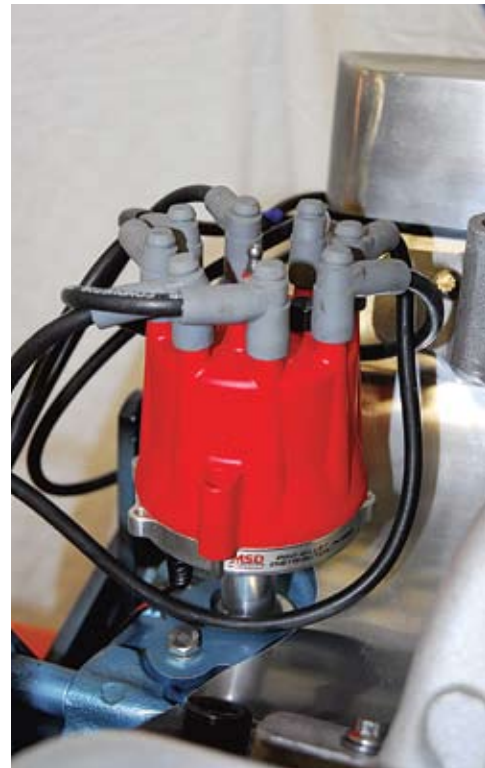
An MSD Pro Billet distributor featuring a TIP prototype polymer distributor gear, locked out mechanical advance, and Taylor wires will handle the spark.
