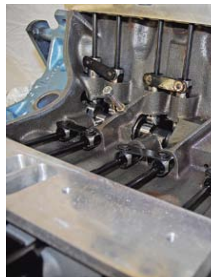
▲ The Comp Cams custom grind solid roller cam features 265/272-degrees duration at 0.050 and 0.691/0.691-inch lift. Crower roller lifters are employed and, though the Comp Cams valvesprings have an open pressure of 620 pounds, Kevin feels that a lifter bore brace isn't needed with this camshaft profile...
