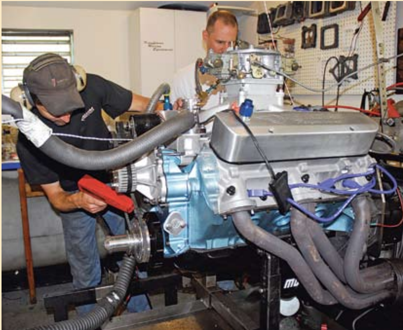
In the dyno cell, the timing is checked on the 463 before a pull is made.
