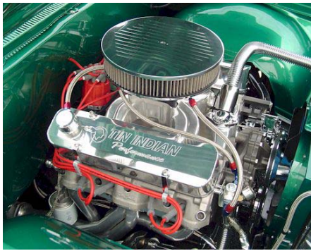
550 HP Street Pump Gas Engine
